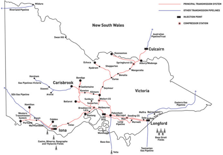
Fig. 2 Victorian gas system: network overview
